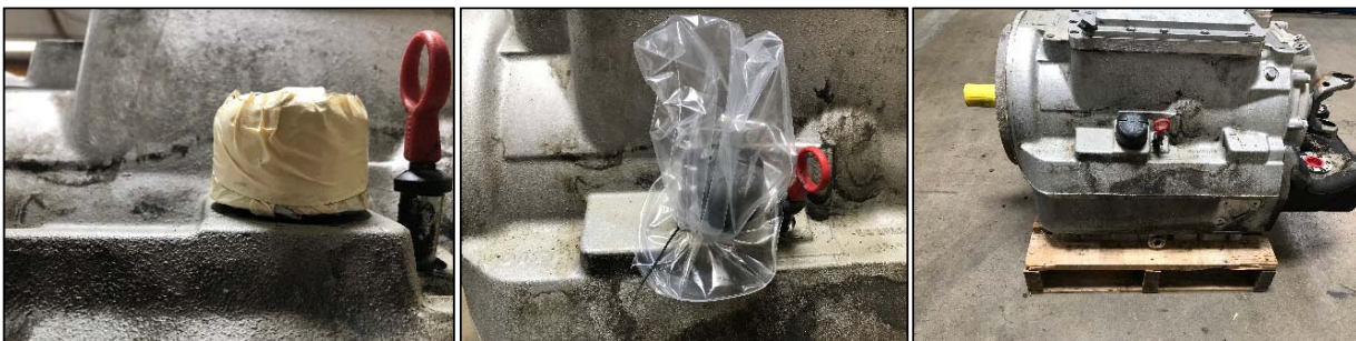
Figure 3.2a—Breather protected from water entry by using tape or plastic and tie strap.
